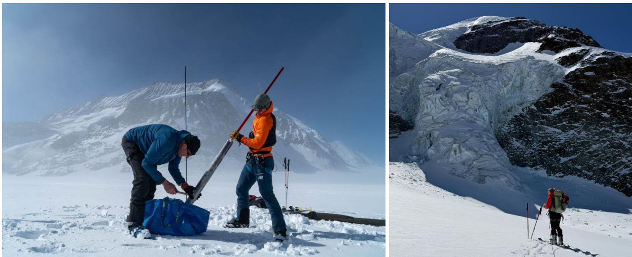
Snow density measurements (Grosser Aletschgletscher, left), and snow depth probing (Vadret Pers, right) in late winter 2026. Photos: L. Hösl / L. van Tricht
