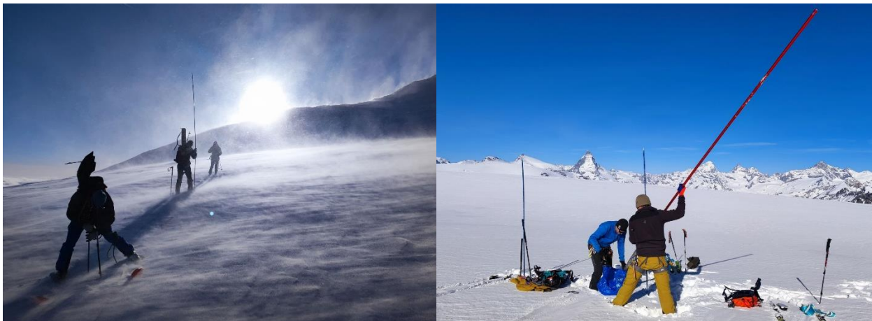
Snow depth probing at 4000 m a.s.l. (Allalingsletscher, left), and snow density measurements (Findelgletscher, right). Photos: M. Huss
