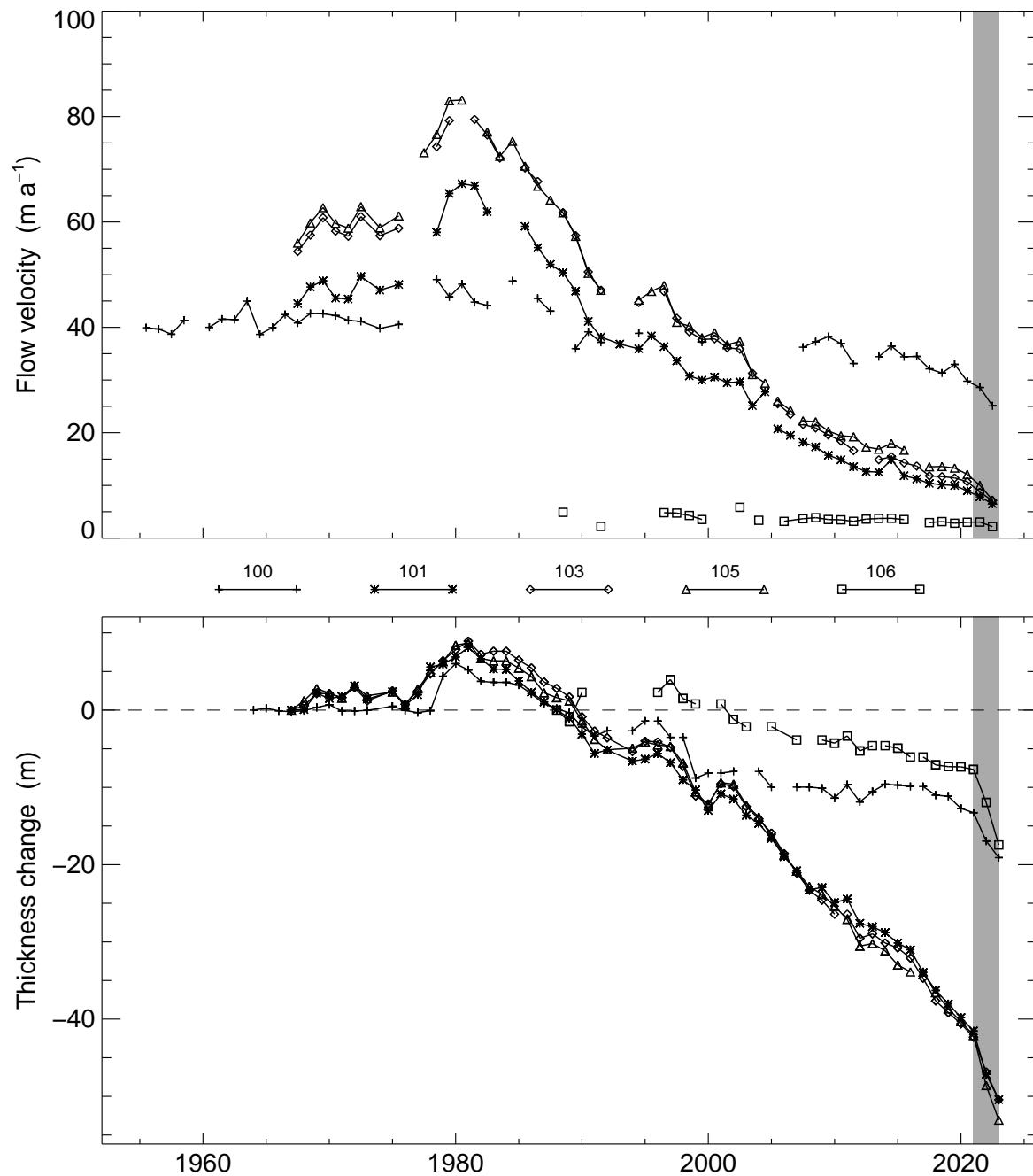
Figure 5.2: Surface flow velocities (top) and thickness change (below) of Allalingletscher at five stakes. The gray-shaded area highlights the years of the current report.
