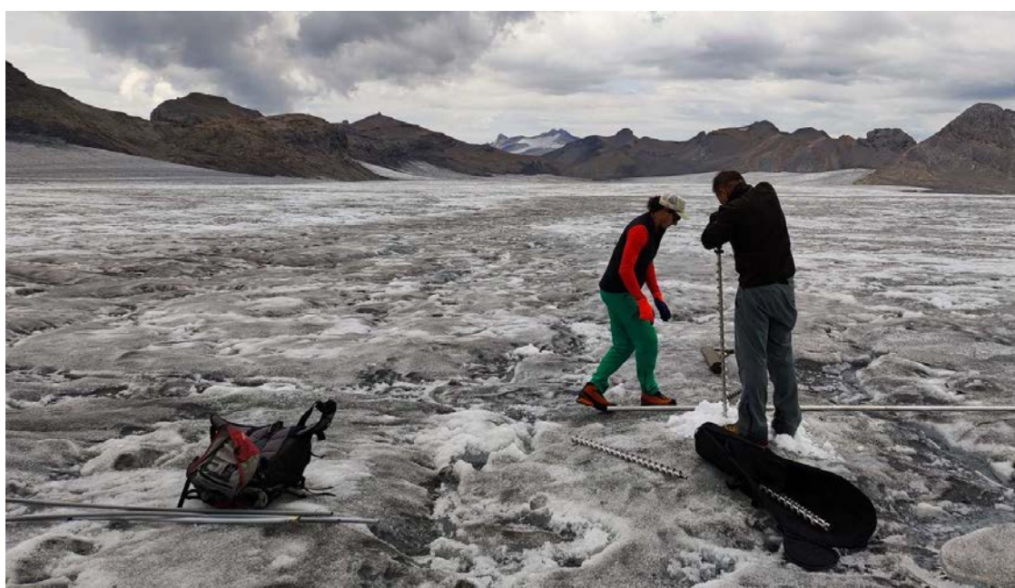
Drilling an ablation stake on the completely snow-free Glacier de la Plaine Morte in August 2022. (Photo: M. Huss)
