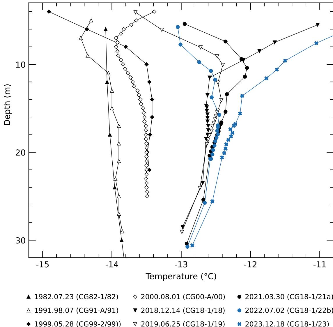
Figure 6.2: Firn temperature profiles at the Colle Gnifetti saddle, measured in 1982 (Haeberli and Funk, 1991), 1991 (Laternser, 1992; Suter et al., 2001), 1999 (Suter, 2002; Suter and Hoelzle, 2002), 2000 (Suter, 2002; Suter and Hoelzle, 2002), 2018/2019 (Mattea et al., 2021), 2021, 2022 and 2023. Most recent measurements of the periods in this report are highlighted in blue. Boreholes CG82-1, CG08-1 are located at the same position while CG91-A and CG00-A are slightly offset to the north-east.
