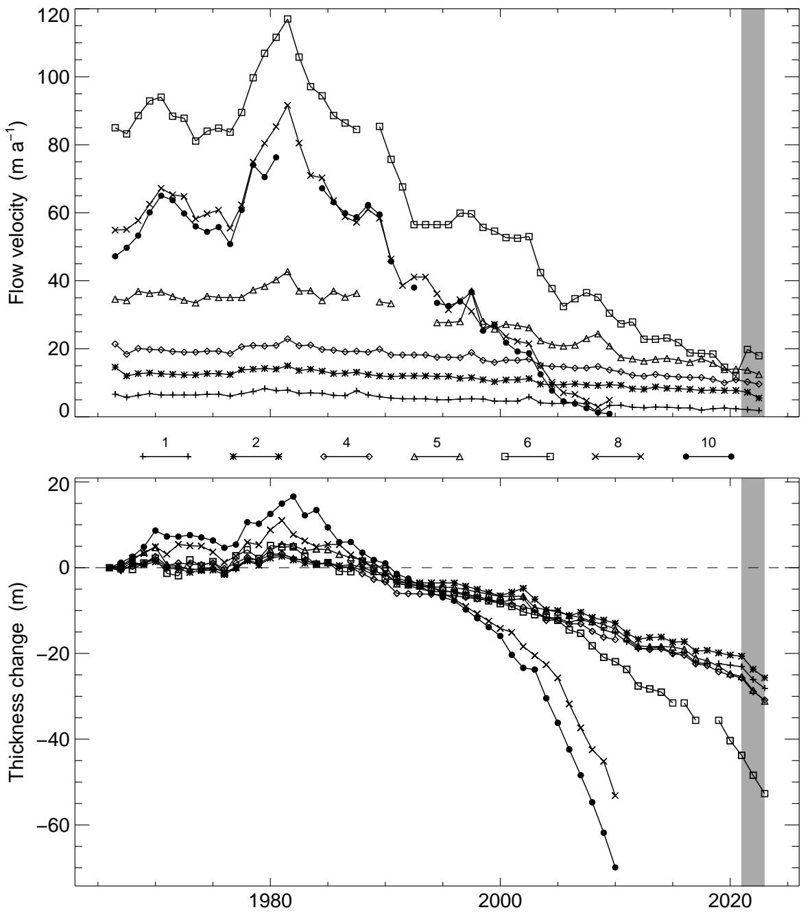
Figure 5.4: Surface flow velocities (top) and thickness change (bottom) of Glacier du Gietro at seven stakes. The gray-shaded area highlights the years of the current report.
