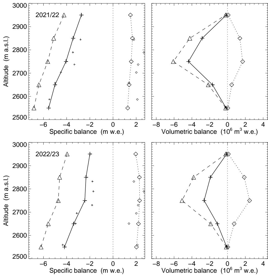
Figure 4.52: Specific (left) and volumetric (right) winter (dotted,  $\diamond$ ), summer (dashed,  $\triangle$ ) and annual (continuous line, +) balance in elevation bands for 2021/22 (top) and 2022/23 (bottom). Small symbols mark the individual measurements.
