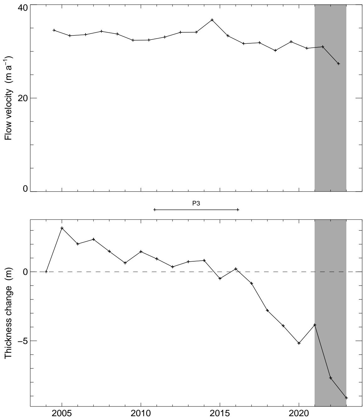
Figure 5.5: Surface flow velocities (top) and thickness change (bottom) at stake P3 on Grosser Aletschgletscher. The gray-shaded area highlights the years of the current report.
