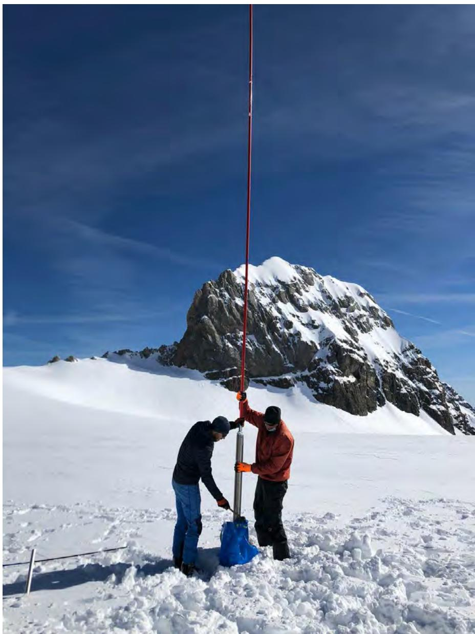
Density measurement using a core drill at the upper site on Claridenfirn in spring 2021
