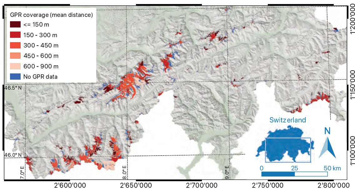
Figure 8.2: Overview of GPR coverage of all glaciers in the Swiss Alps. Available thickness measurements are color-coded indicating the mean of the distance of all grid points on a glacier to the closest thickness measurement. Glaciers with no direct thickness measurements are shown in blue.
