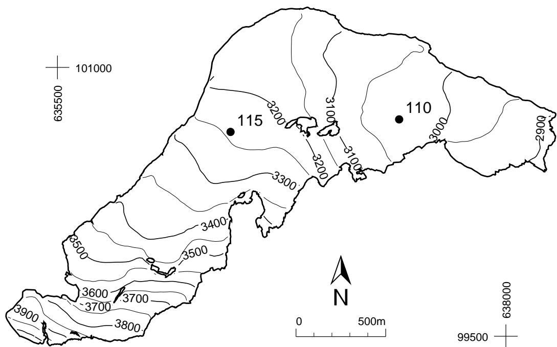
Figure 4.26: Surface topography and observational network of Hohlaubgletscher.
