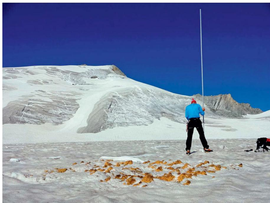
Marked horizon of the previous summer surface that melted out completely on Rhone-gletscher at stake 3 in September 2018 (Photo: M. Huss)
