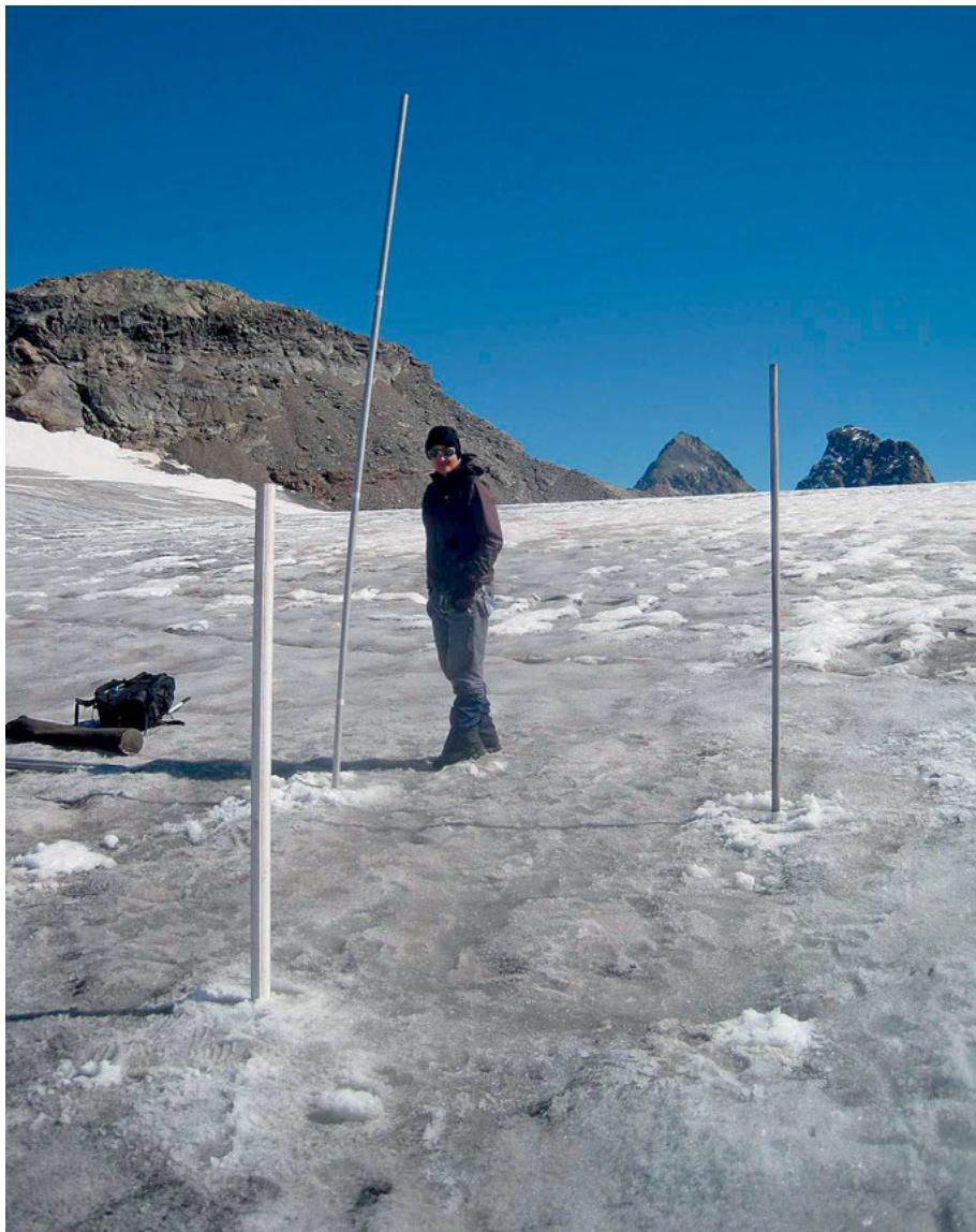
Experiment with stakes of different material: plastic, aluminum and wood (Photo: A. Bauder)
