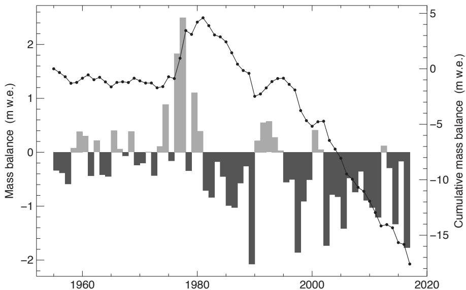
Figure 5.10: Schwarzberggletscher - Mean specific annual balance (bars) and cumulative mass balance (line) for the period 1955-2017.
