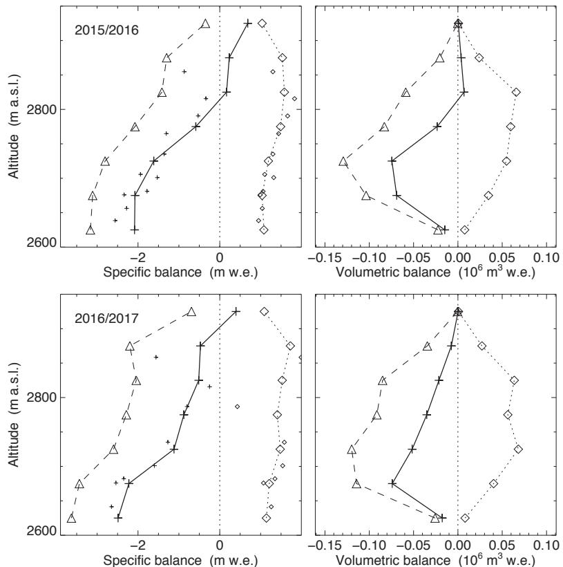
Figure 4.27: Specific (left) and volumetric (right) winter (dotted,  $\diamond$ ), summer (dashed,  $\triangle$ ) and annual (continuous line, +) balance versus altitude for 2015/16 (top) and 2016/17 (bottom). Small symbols mark the individual measurements.
