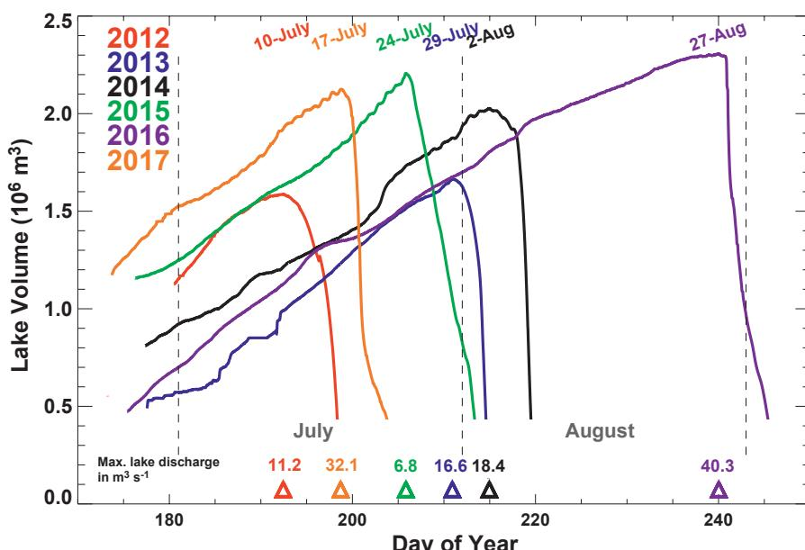
Figure 6.6: Temporal evolution of water volume at Lac des Faverges between 2012 and 2017. The date of the outburst event and the maximum lake discharge are given.
