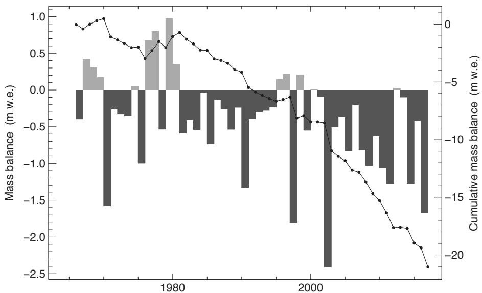
Figure 5.4: Glacier du Gietro - Mean specific annual balance (bars) and cumulative mass balance (line) for the period 1966-2017.
