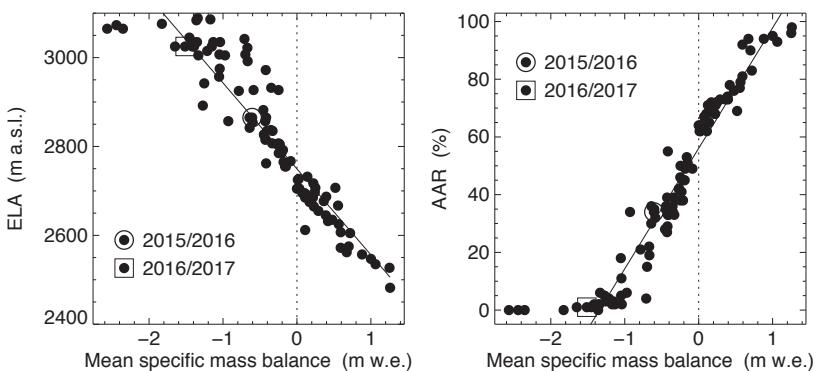
Figure 4.31: Equilibrium line altitude (ELA) and accumulation area ratio (AAR) versus mean specific balance including all previous observations.
