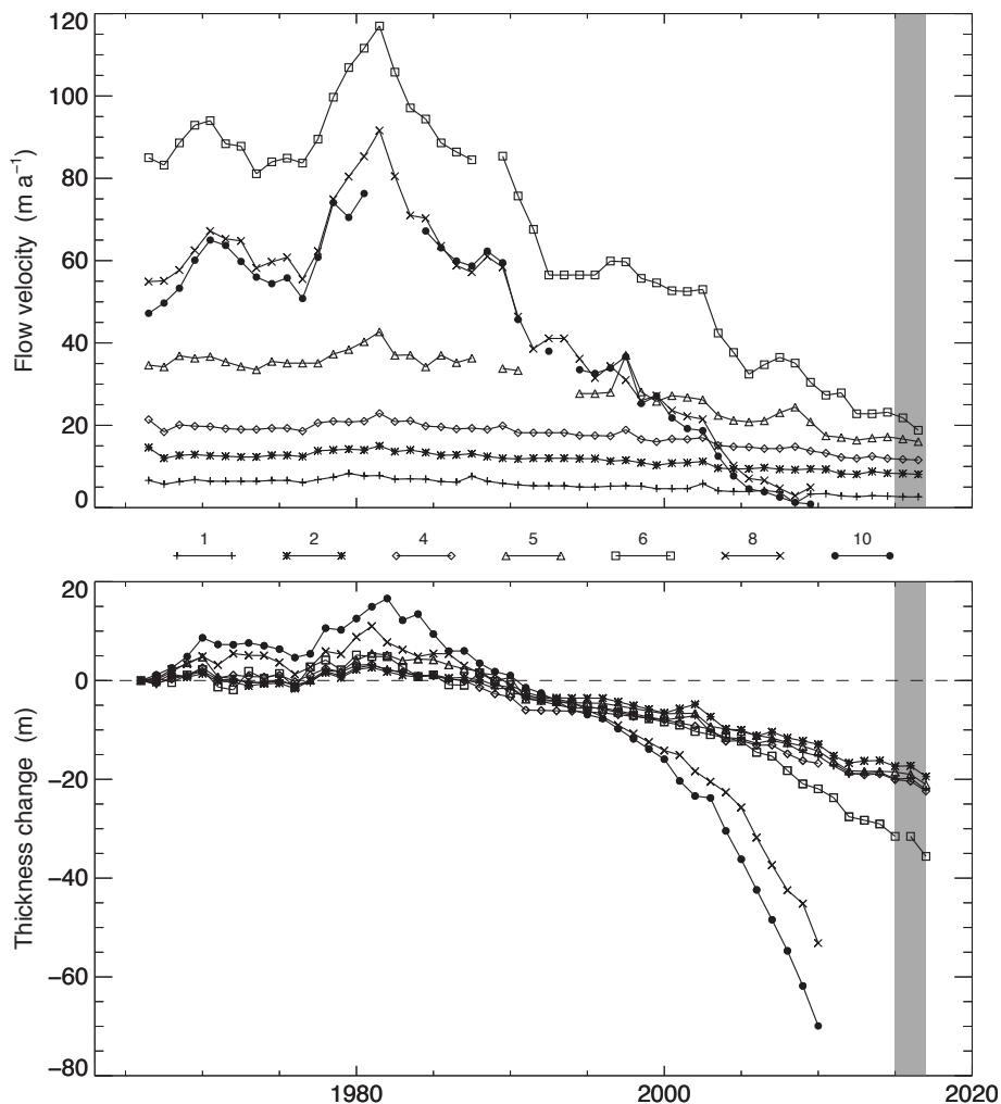
Figure 5.3: Surface flow velocities (top) and thickness change (bottom) of the Glacier du Giétra at all seven stakes. The gray shaded area highlights the years of the current report.
