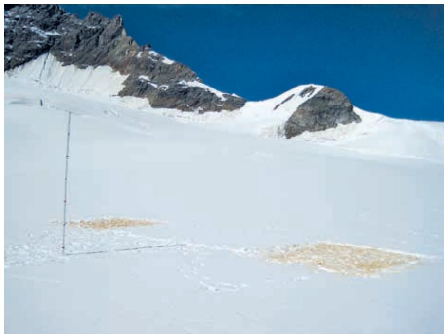
Stake P3 on Jungfraufirn in September 2016 with two marked patches for locating the reference surface during measurements in the subsequent year (Photo: A. Bauder)
