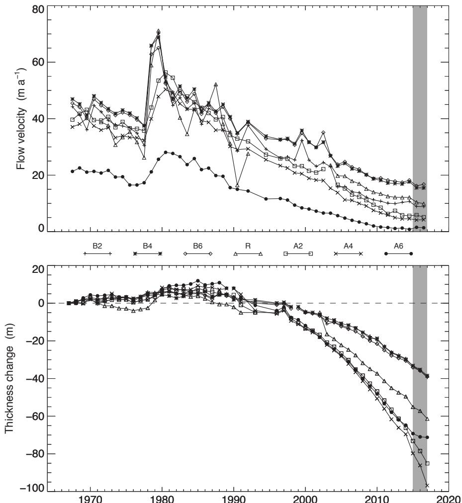
Figure 5.6: Surface flow velocities (top) and thickness change (bottom) of the Glacier de Corbassière at two profiles with three stakes each and the additional stake in between. The gray shaded area highlights the years of the current report.
