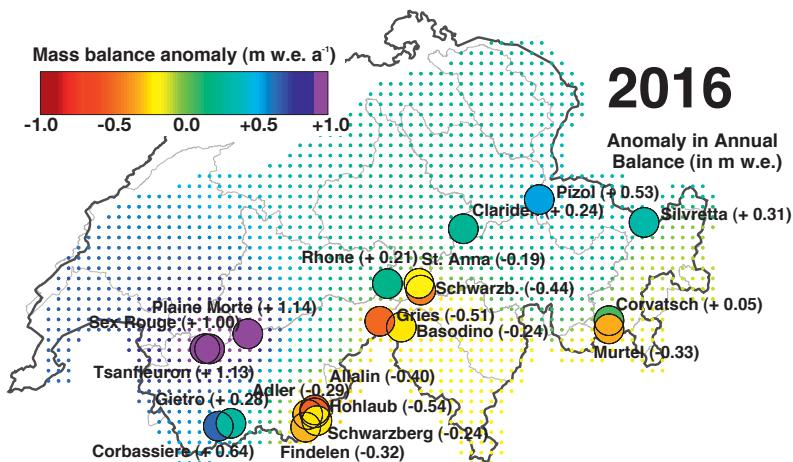
Figure 4.38: Anomaly in annual surface mass balance in the 2015/16 hydrological year relative to the average 2005/06 to 2014/15 period for all observed glaciers and extrapolated to the entire Swiss Alps.
