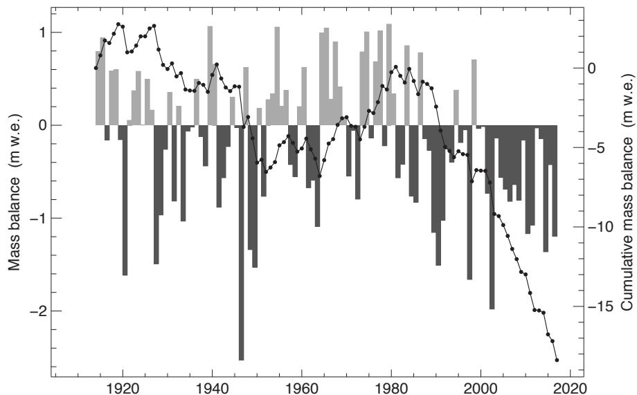
Figure 4.36: Claridenfirn - Mean specific annual balance (bars) and cumulative mass balance (line) for the period 1914-2017.
