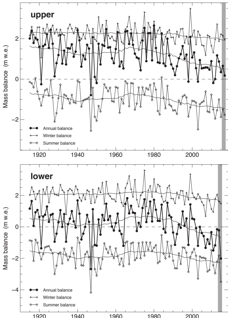
Figure 4.35: Mass balance of the upper (top) and lower (bottom) stake on Claridenfirn over the whole observation period. The gray shaded area highlights the years of the current report.
