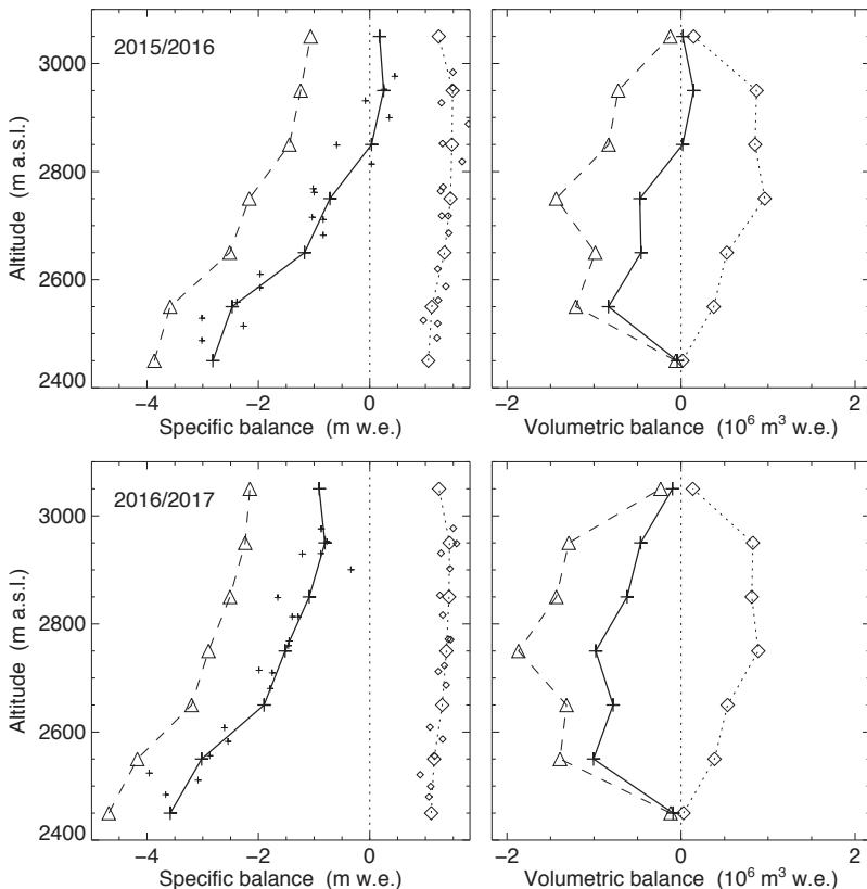
Figure 4.30: Specific (left) and volumetric (right) winter (dotted,  $\diamond$ ), summer (dashed,  $\triangle$ ) and annual (continuous line, +) balance versus altitude for 2015/16 (top) and 2016/17 (bottom). Small symbols mark the individual measurements.
