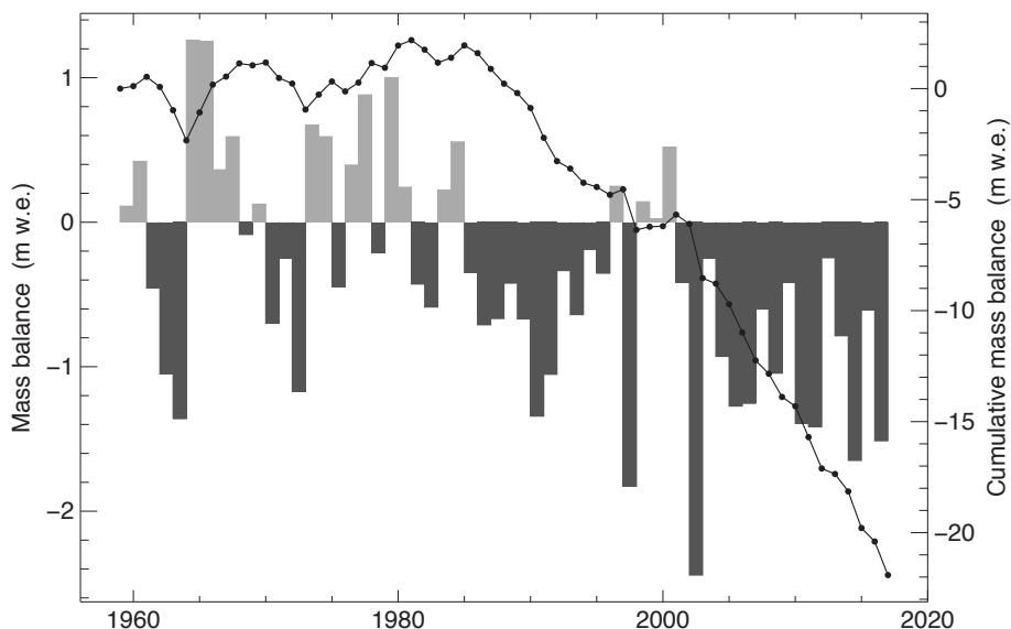
Figure 4.29: Silvrettagletscher - Mean specific annual balance (bars) and cumulative mass balance (line) for the period 1959-2017.
