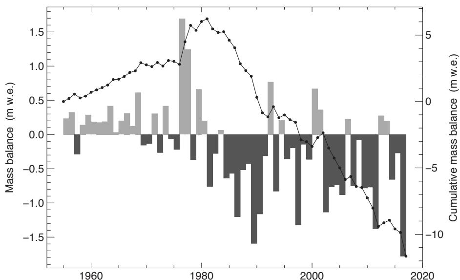
Figure 5.9: Allalingletscher - Mean specific annual balance (bars) and cumulative mass balance (line) for the period 1955-2017.
