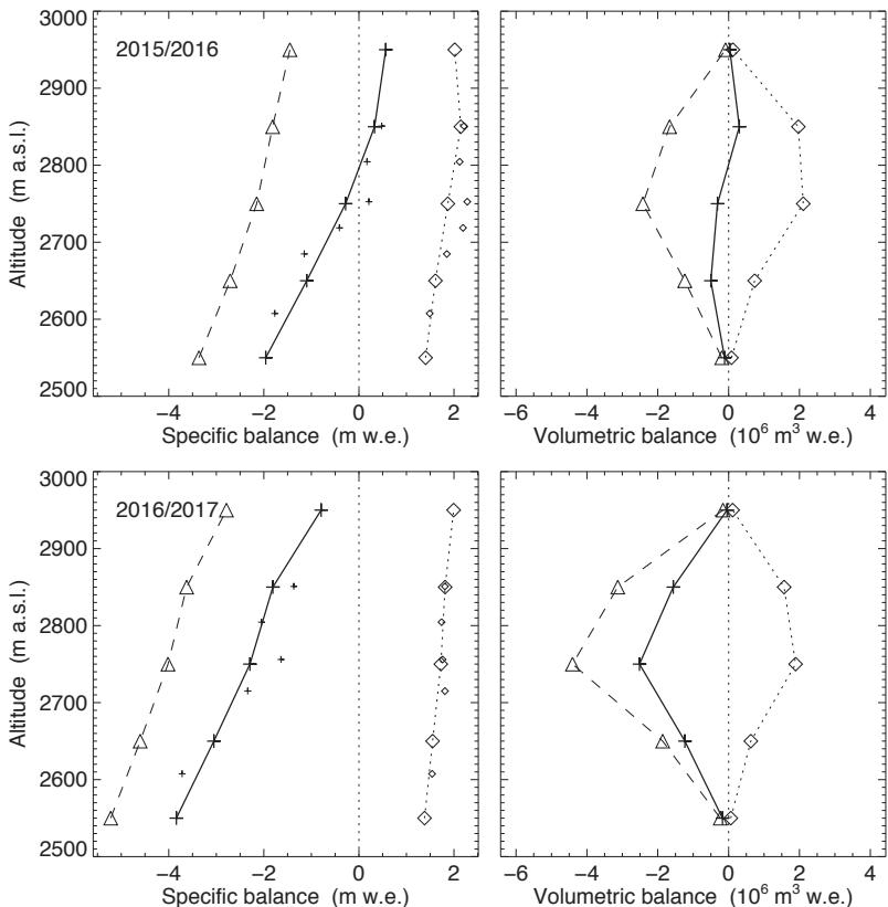
Figure 4.33: Glacier de Tsanfleuron - Specific (left) and volumetric (right) winter (dotted,  $\diamond$ ), summer (dashed,  $\triangle$ ) and annual (continuous line,  $+$ ) balance versus altitude for 2015/16 (top) and 2016/17 (bottom). Small symbols mark the individual measurements.
