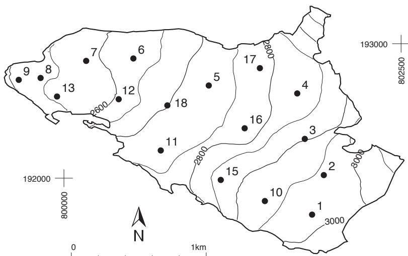
Figure 4.28: Surface topography and observational network of the Silvrettagletscher.
