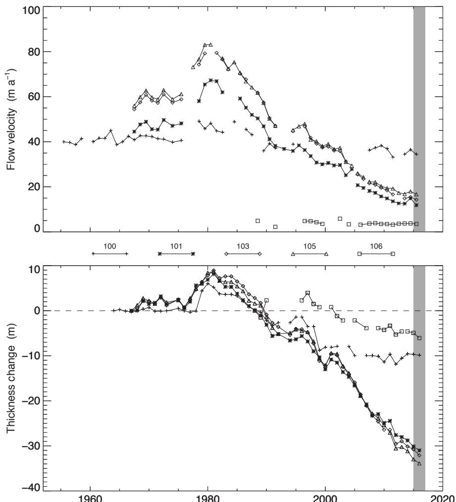
Figure 5.8: Surface flow velocities (top) and thickness change (below) of the Allalingletscher at five stakes. The gray shaded area highlights the years of the current report.
