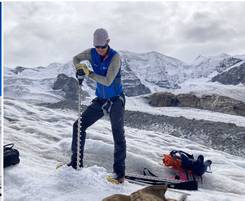
(Left) Snow density measurements on Grosser Aletschgletscher in late March 2025. Photo: M. Huss. (Right) Drilling of an ablation stake on Vadret Pers in September 2025. Photo: A. Linsbauer.
