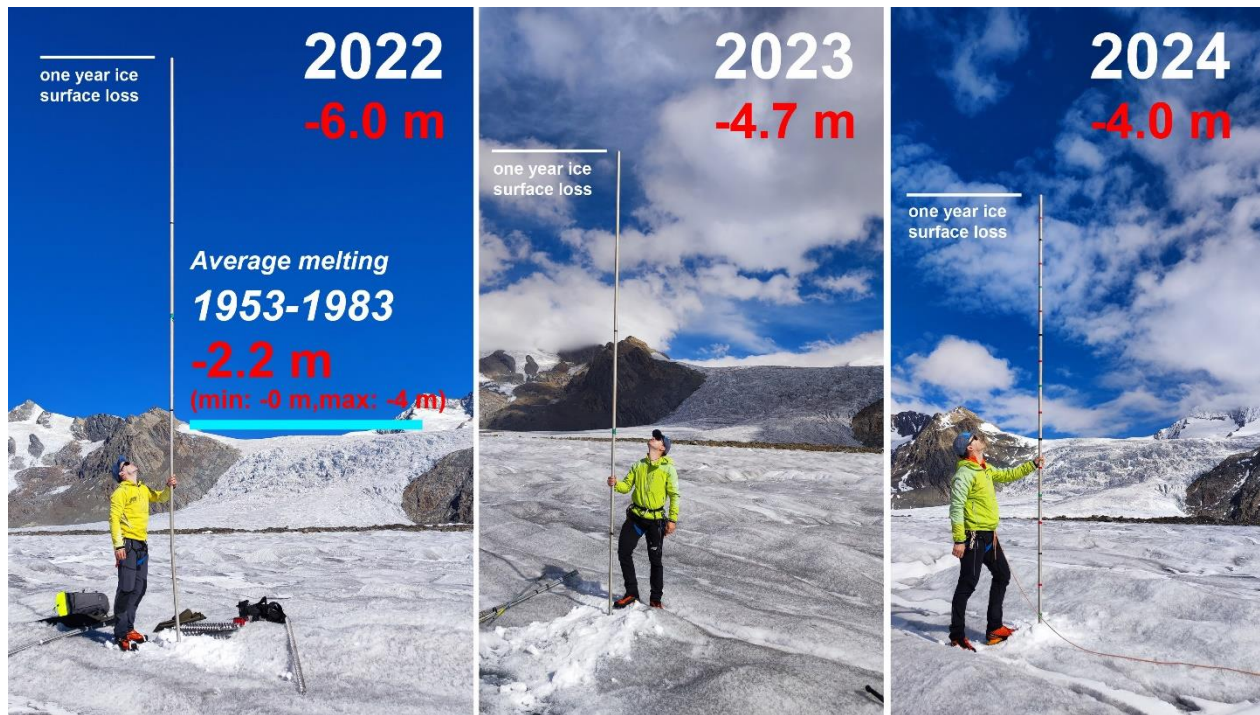
Glacier mass balance measurement stake at Konkordiaplatz (2650 m a.s.l.), Grosser Aletschergletcher. Comparison of the observed melt rate in 2024 (right) with the extreme years 2022 and 2023, and the average from the observations performed in 1953-1983. Photos: M. Huss
